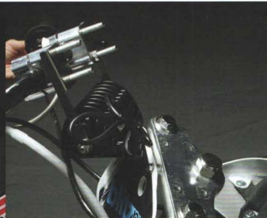
Install the headlight with brackets by lining it up with the four stem bolts
