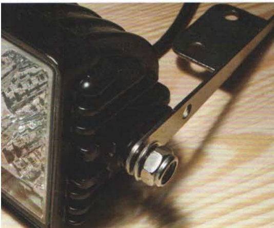
Begin first by installing the brackets onto the light with the tabs pointing inwards
