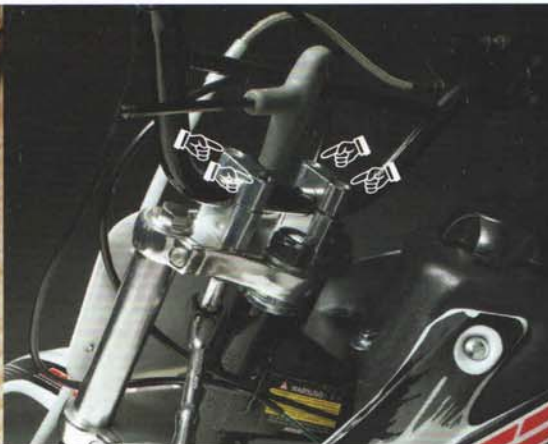
Remove the four stem bolts carefully by turning the fork to access the bolts
