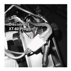
**Step five:** Find the cloth strap inside the controller box that is attached to the battery (see pic below). Slowly pull on the cloth strap; you might have to pull a bit hard to slide the battery out. If the battery does not want to come out the tube might be out of round. Check to see tube is damaged.
