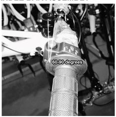
Attach the handlebars as shown. There are 4 screws to assemble or remove the handlebar. The Power S/W should be at a 60-90 degree angle, pointing straight up. This allows the small riders to twist the throttle all the way open.
