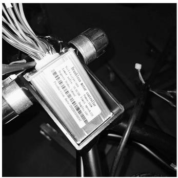
Push the controller into the box. Make sure the charging wire does not get smashed.
