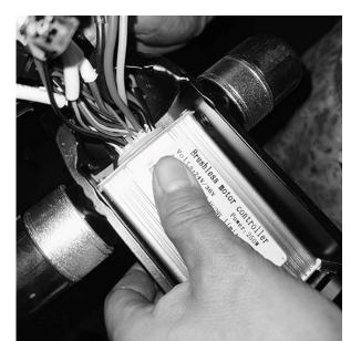
Plug in the XT-60 connector and wrap the wire protector around it. Tuck all the wires in and plug in the speed switch. When you are done it should look like the pic below.
